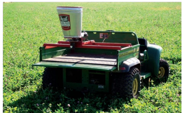
Broadcast seeder mounted on a utility vehicle.
